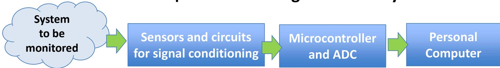
Identification of key physical quantities (temperature, humidity, force, acceleration, speed, ...)
